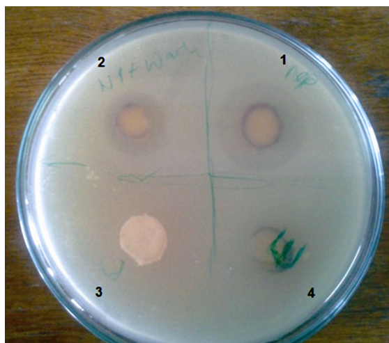
Fig. 4—Antibacterial activity of silver nanoparticles 1 & 2 test samples and 3 & 4 are controls
