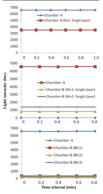
Fig.2 — Light cutting ability of different fabrics
