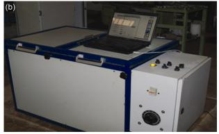
Fig.1 — (a) Line diagram of instrument and (b) photograph of instrument to determine heat and light cutting ability of curtain
