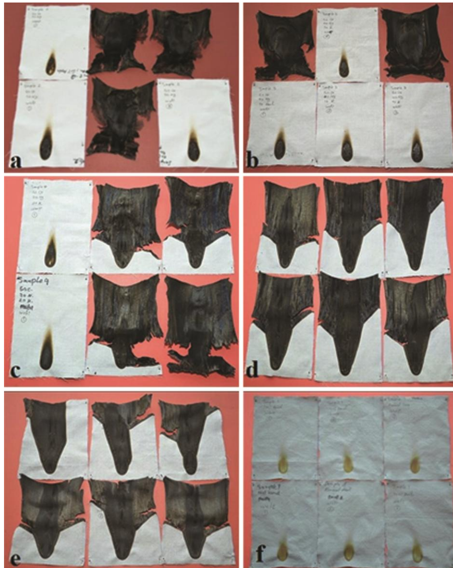
Fig. 3—Images of cotton/nylon-Kermel blended fabric samples [(a) Sample 1 (Co50/Ny50), (b) Sample 2 (Co50/Ny40/K10), (c) Sample 3 (Co50/Ny30/K20), (d) Sample 4 (Co50/Ny20/K30), (e) Sample 5 (Co50/Ny10/K40) and (f) Sample 6 (K100)]
