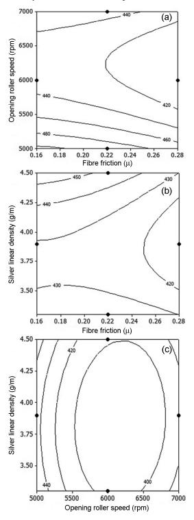
Fig. 3—Effects of (a) fibre friction with opening roller speed, (b) fibre friction with sliver linear density and (c) opening roller speed with sliver linear density on yarn imperfections
