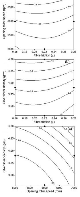
Fig. 4—Effects of (a) fibre friction with opening roller speed, (b) fibre friction with sliver linear density and (c) opening roller speed with sliver linear on yarn hairiness index (H)
