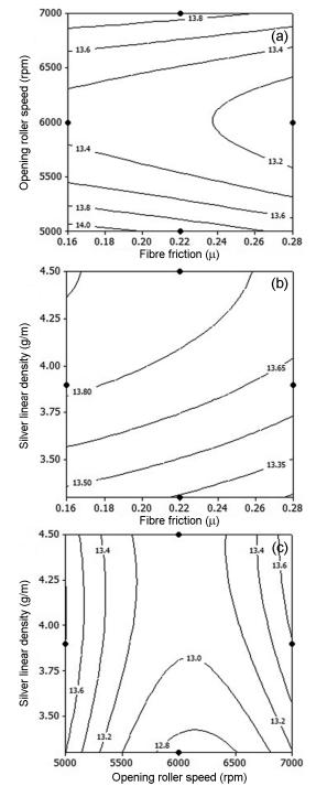
Fig. 1—Effects of (a) fibre friction with opening roller speed, (b) fibre friction with sliver linear density and (c) opening roller speed with sliver linear density on yarn tenacity
