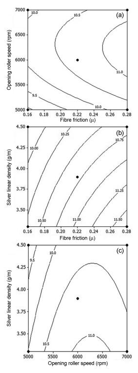
density of 3.92 g/m. It is evident from the contour that an increase in fibre friction decreases the yarn imperfections due to controlled flow of fibres in the transport channel and deposition of more or less equal number of fibres in the rotor groove.
