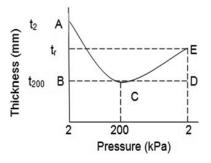
Fig. 2 — Typical thickness-pressure curve for textile floor coverings (Source: BS 4098: 1975)
