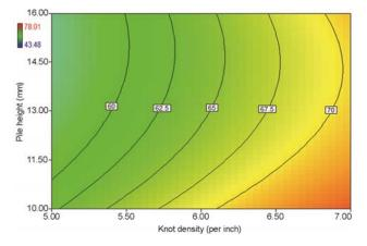
Fig. 5 — Effect of knot density and pile height on per cent compression recovery
