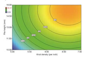
Fig. 4 — Effect of knot density and pile height on compression
