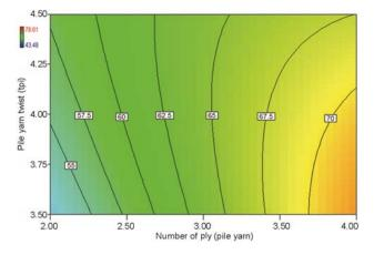
Fig. 7 — Effect of number of ply in pile yarn and pile yarn twist on per cent compression recovery
