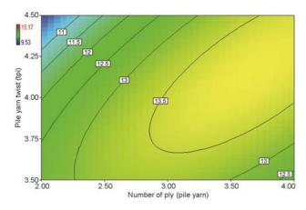
Fig. 6 — Effect of number of ply in pile yarn and pile yarn twist on compression
