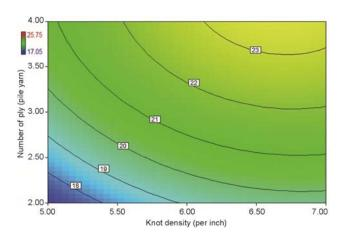
Fig. 3 — Effect of knot density and number of ply in pile yarn on carpet thickness at 2 kPa
