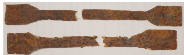
Fig. 1 — Ruptured composite samples after tensile testing
