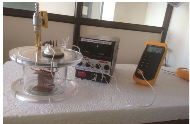
Fig. 2 — Experimental setup for calculation of thermoelectric power.
