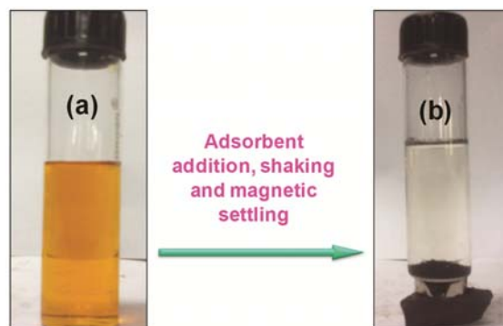
Fig. 11 – Adsorption of methyl orange (MO) dye using \text{Fe}_3\text{O}_4@\text{AC} NC containing ~22 wt % of oleic acid capped \text{Fe}_3\text{O}_4 nanoparticles (FAC4) followed by magnetic separation of spent adsorbent particles.
