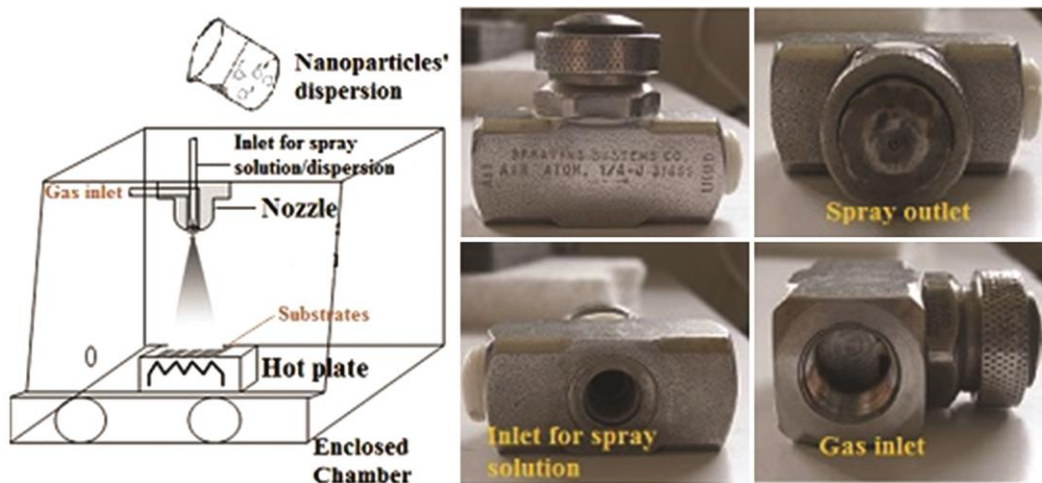
Fig. 3 — A schematic of the spray apparatus used to deposit compact \text{TiO}_2 films. The photographs depict the solution and gas inlets, and also the spray outlet of the nozzle.
