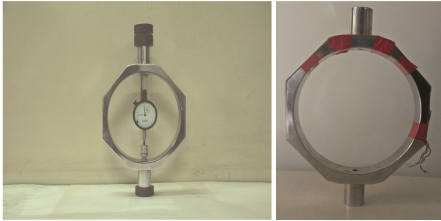
Fig. 5 — A dial gauged and strain gauged octagonal ring shaped force transducer.
