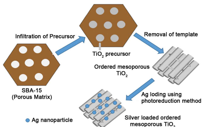
Fig. 1 — Schematic illustration of the synthesis of SMTO material.
