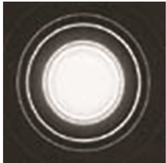
Fig. 3 — An example of SAED pattern of thermally evaporated aluminium film.
