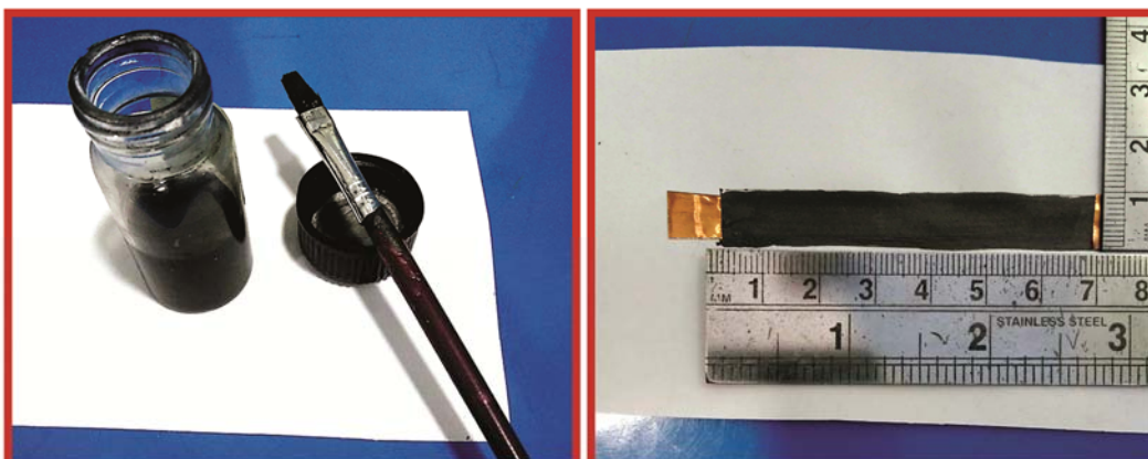
Fig. 2 – (a) Graphene ink and (b) schematic structure of graphene based piezoresistive strain sensor where graphene is used as sensing material.
