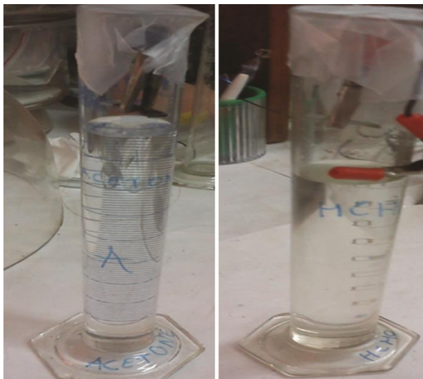
Fig. 1 — Experimental set up of exposure of CdTe thin film to acetone and formaldehyde vapors.
