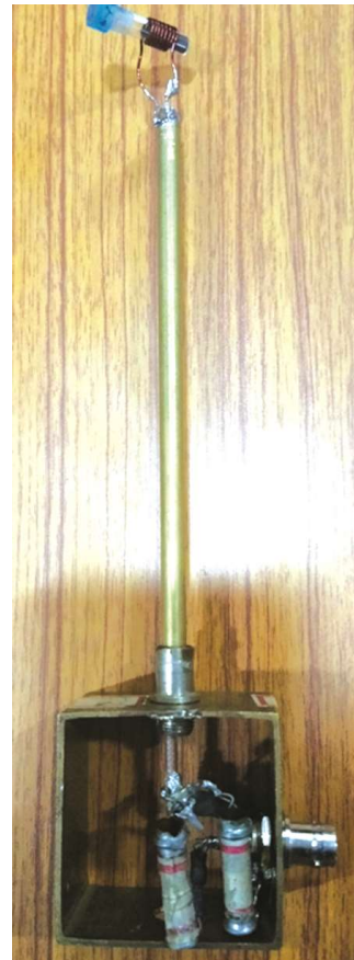
Fig. 4 — Home-made low temperature probe.
