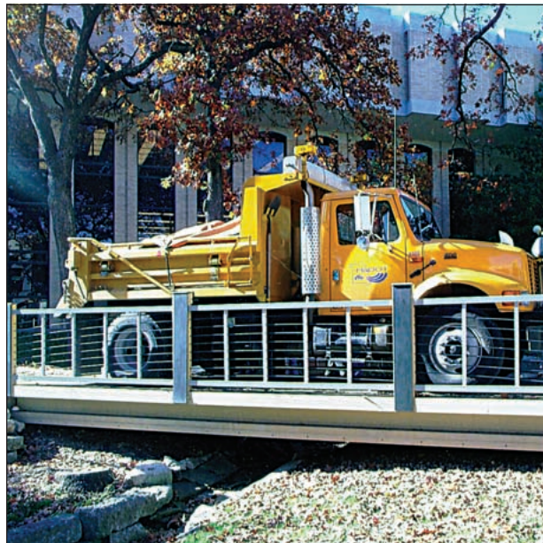
Fig. 3. UMR smart composite bridge during a near-rating load test with a weighted truck.
