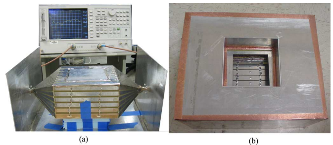
Fig. 3. Modified TEM cell. (a) Without absorbing materials and shielding box. (b) Complete cell.
