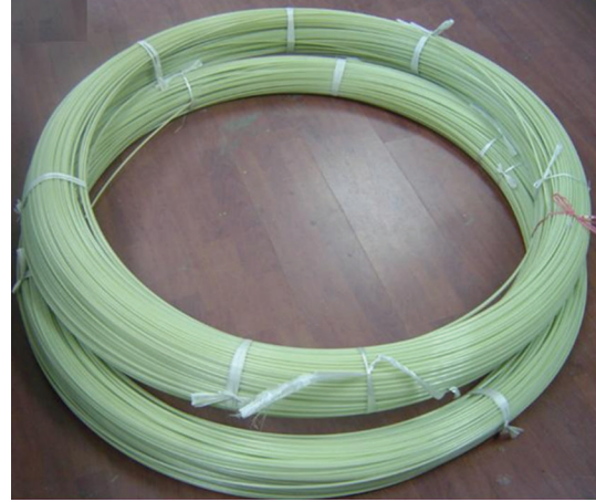
FIGURE 1: Finished product of FRP-OF bars.
