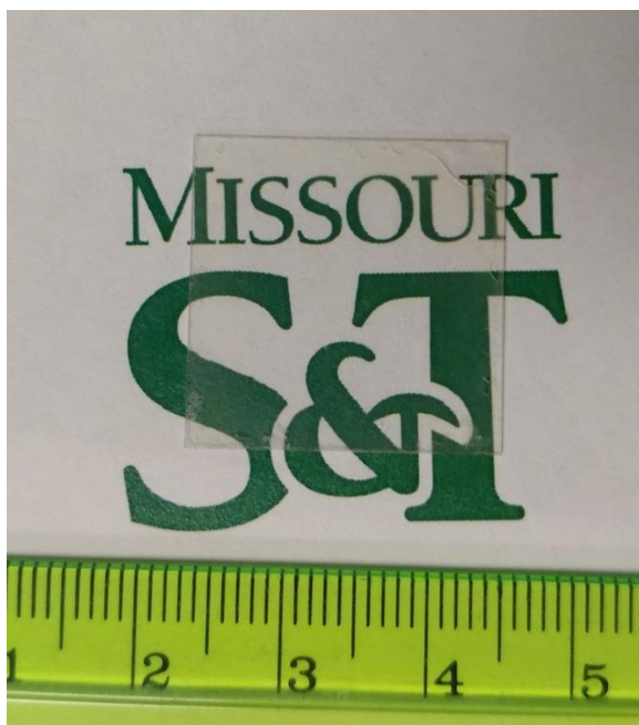
Figure 12. Specimen bonded with CMH liquid precursor at 67 °C.
