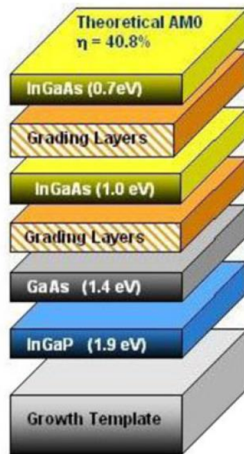
Figure 1.1. Schematic of IMM cross-section before inversion, illustrating differences in band gap energies between semiconductor layers 1 .
