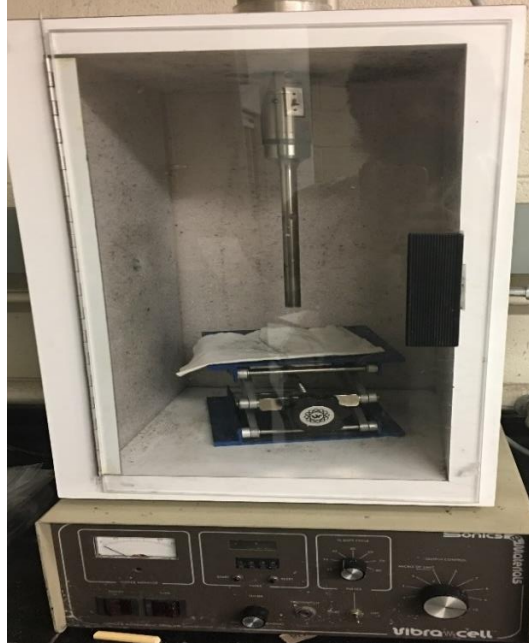
Figure 5.1. Vibra-cell sonicator for stabilizing nanoparticle suspensions.
