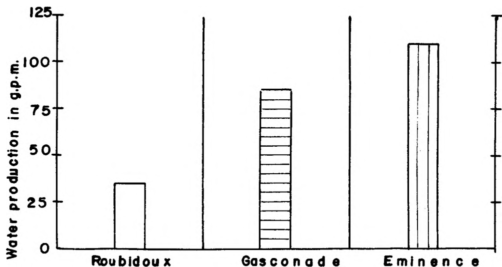
MAXIMUM WATER PRODUCTION FROM THE WELLS COMPLETED IN THE RB., GC., AND EM. FORMATIONS
