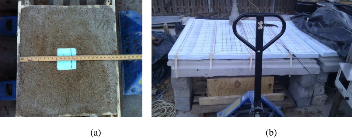
Figure 2.22 (a) Large sandbox and piece of construction foam to simulate void and (b) placed behind the MSE wall section using a pallet jack
