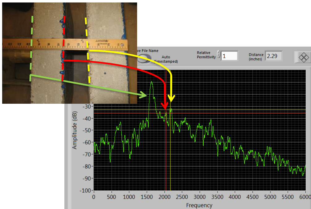
Figure 2.7 Testing the 8-18 GHz FM-CW radar on two concrete slabs in the laboratory
