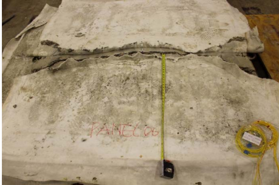
Fig. 6.16. Cracks in P6 after load frame test.
