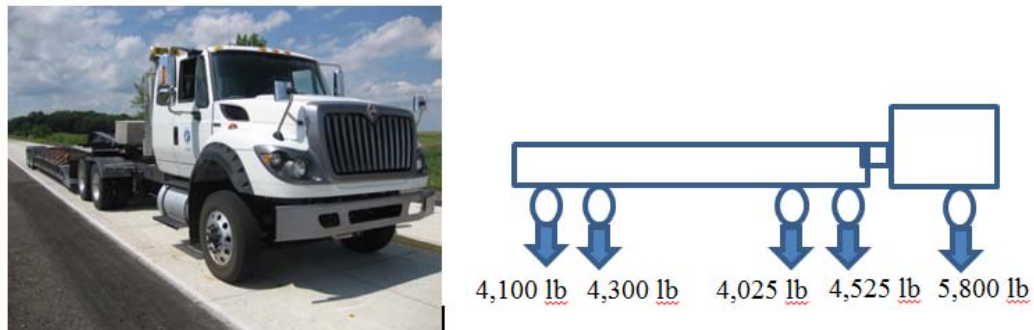
Fig. 7.4. Photos for overlay after paving, truck and truck dimensions.
