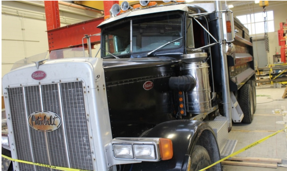
Fig. 5.1. Dump truck used to load concrete panels.
