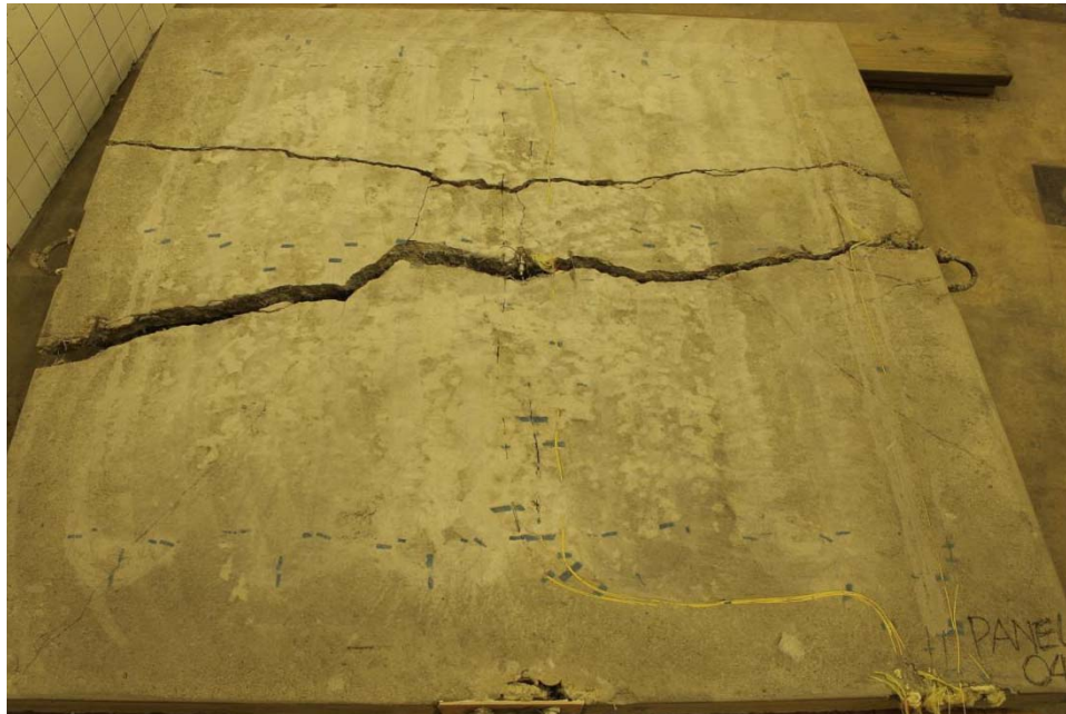
Fig. 6.13. Cracks in P4 after load frame test.
