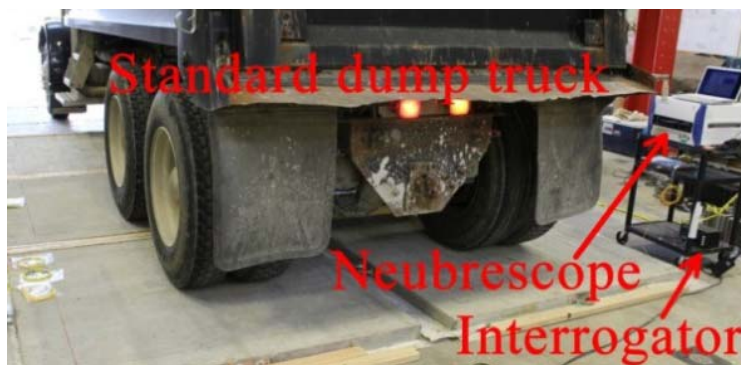
Fig. 5.4. Concrete panels under truck loads.
