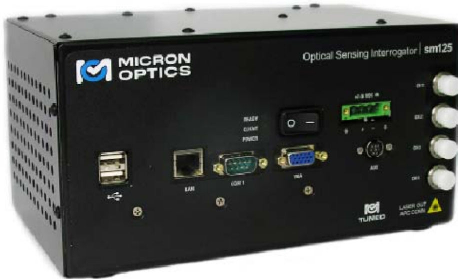
Fig. 2.2. Optical sensing interrogator sm125.
