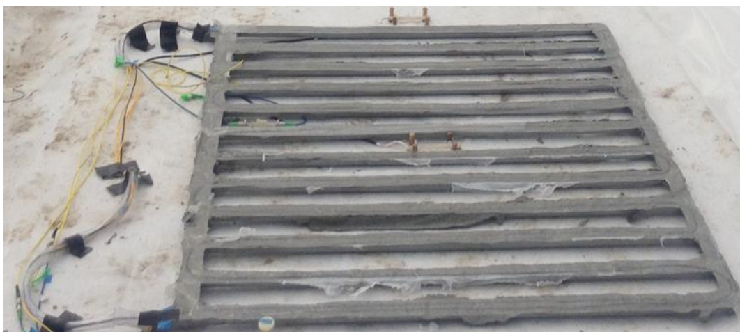
Figure 3.5 A smart grid laid on top of fabric sheet
