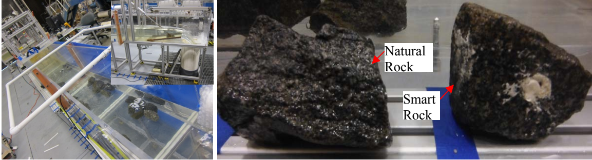
(a) Small Flume at TFHRC (b) Natural Rocks with and without an Embedded Magnet Figure 3.23 Overview of the Small Flume and a Passive Smart Rock
