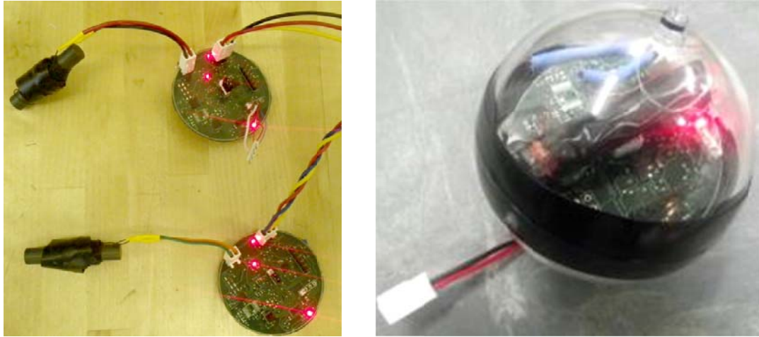
(a) v2.5 Board with Attached Ferrite-core Antennas (b) Board in a Plastic Shell
