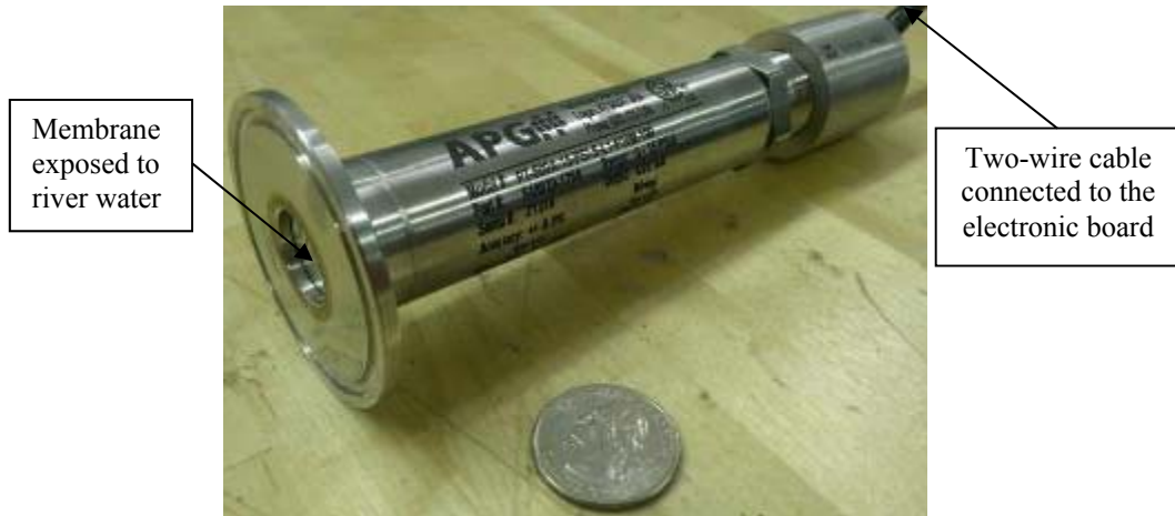
Figure 4.36 An APG PT-500 Pressure Sensor
