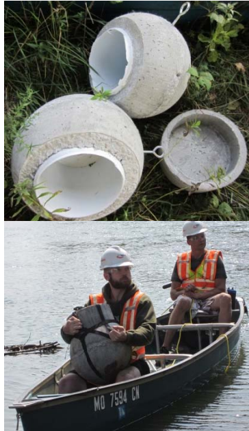
(a) Active Smart Rocks Deployed
