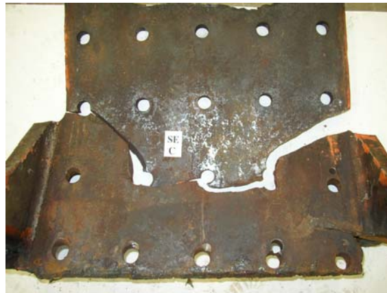
Figure 1.8 Fracture Pattern of SE Strut Web
