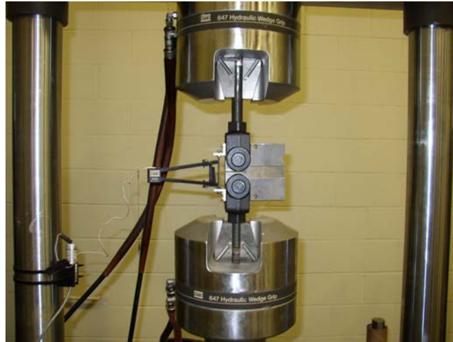
Figure 6.4 Crack Growth Test Set-up
