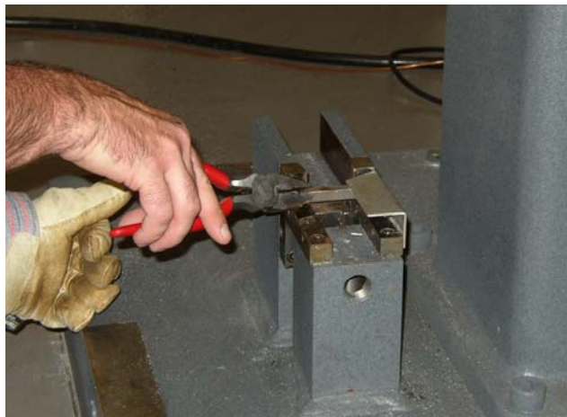
Figure 5.5 Placing Charpy V-Notch Specimen in Anvil
