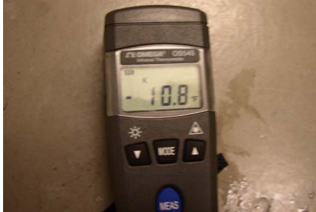
Figure 5.4 Temperature as Measured from Alcohol Bath
