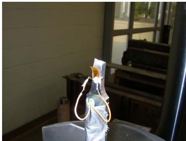
Figure 4.4 Failure of Fatigue Specimen
