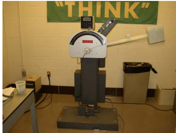
Figure 5.2 Tinius Olsen Model 84 Universal Impact Tester
