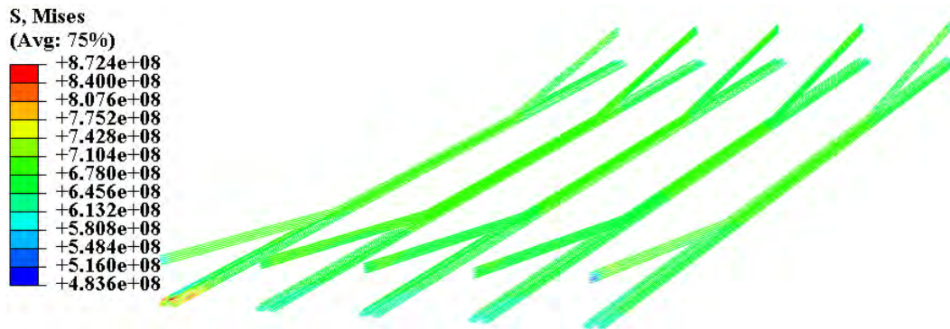
Fig. 3.9 Von Mises stress in prestressed tendons. ( \times 10 ).
