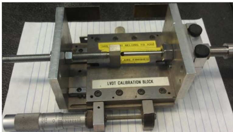
Figure 7.6: Calibration of a DC-LVDT with calibration block
