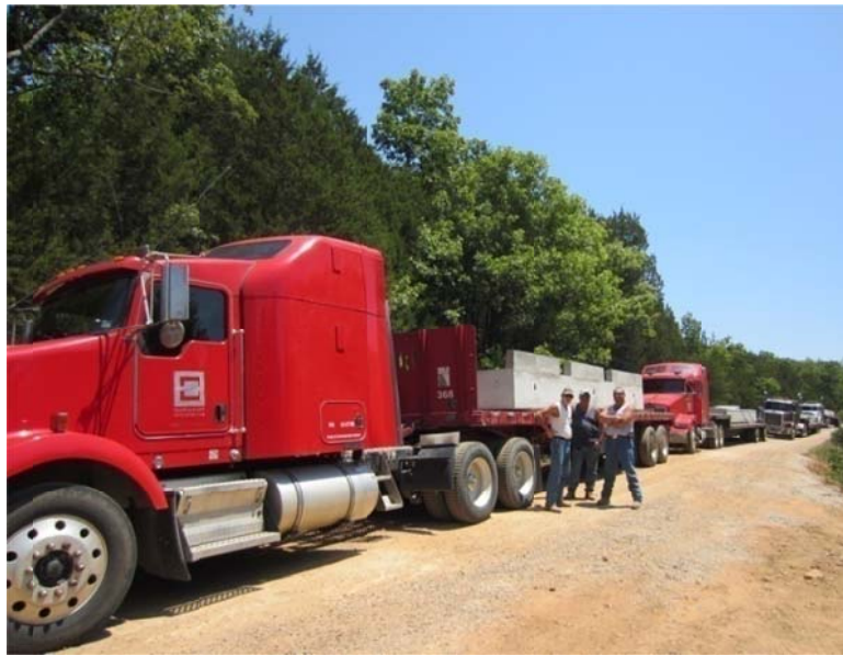
Figure 5.9: Transportation of precast bridge elements
