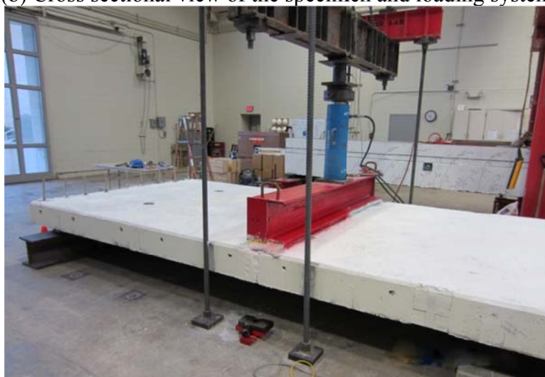
(c) Overview of the loading system
