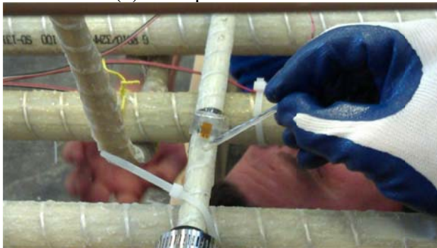
(d) Apply some resin on the smooth surfaces (e) Fold back and press down the gauges with foam
