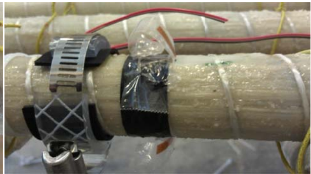
(a) Position each gauge by taping down lead wires (b) Fold up free end of the strain gauges
