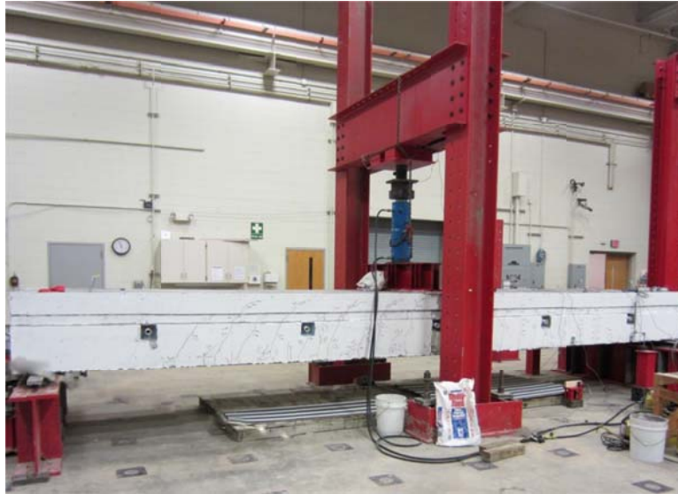
(a) Overview of the crack pattern
