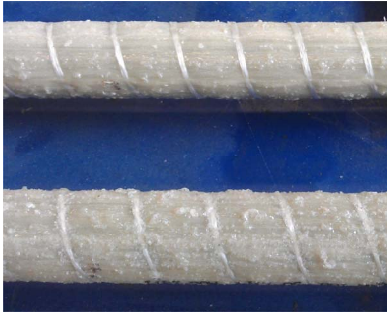
(a) Wrapped and sand-coated Aslan 100 GFRP-bars
