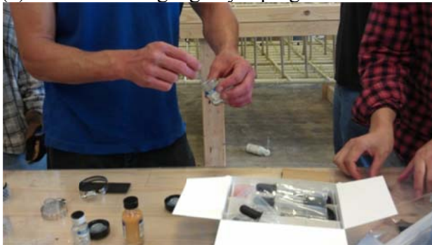
(c) Stir up resin for about 5 minutes and let it set for another 5 minutes
