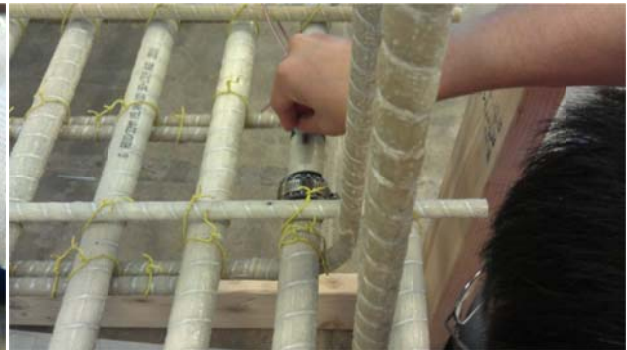
(d) Apply some resin on the smooth surfaces (e) Fold back and press down the gauges with foam
