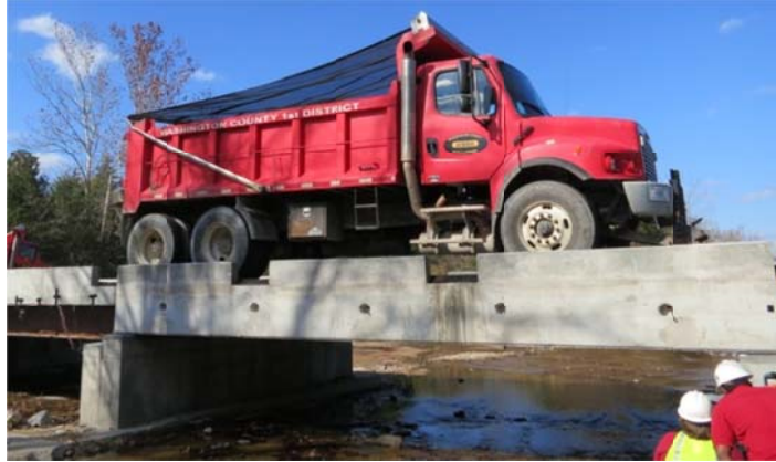
(a) Fully loaded dumb truck (44 kips total)
