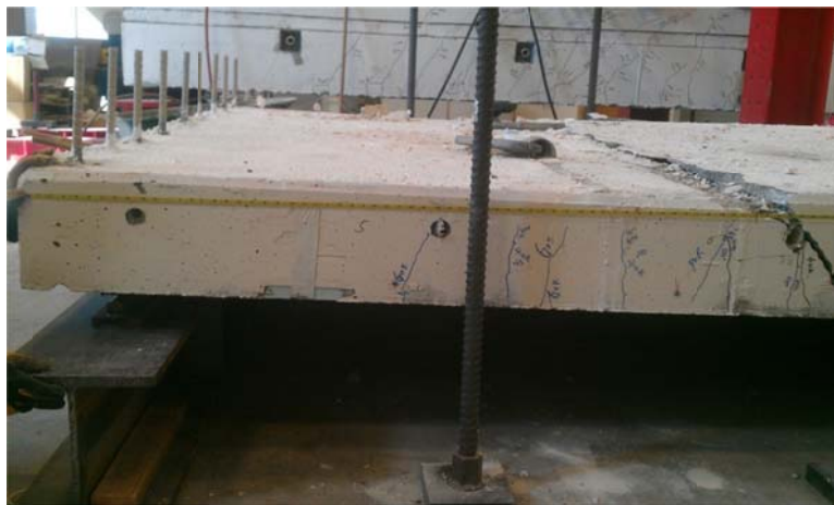
Figure 7.19: Slab failure by shear
