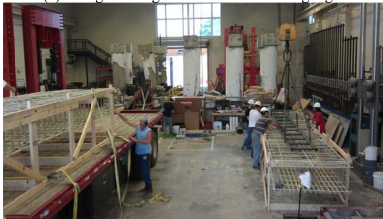
(b) Loading and unloading of GFRP-bar cages
