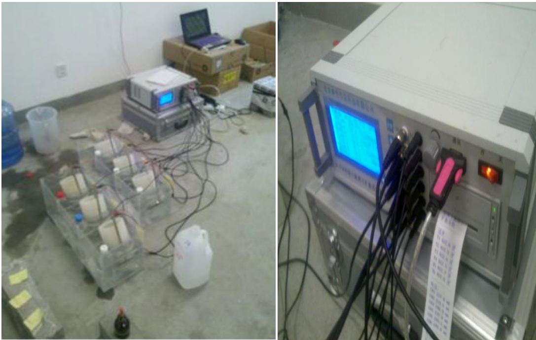
Figure 4.5 Chloride Penetration Test Setup
