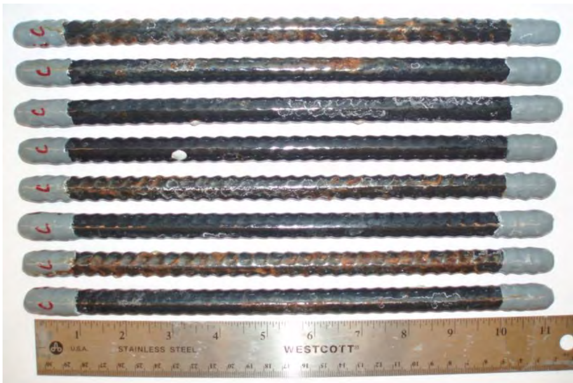
Figure A - 19: Left side of the deformed pure enamel-coated salt spray specimens after testing.
