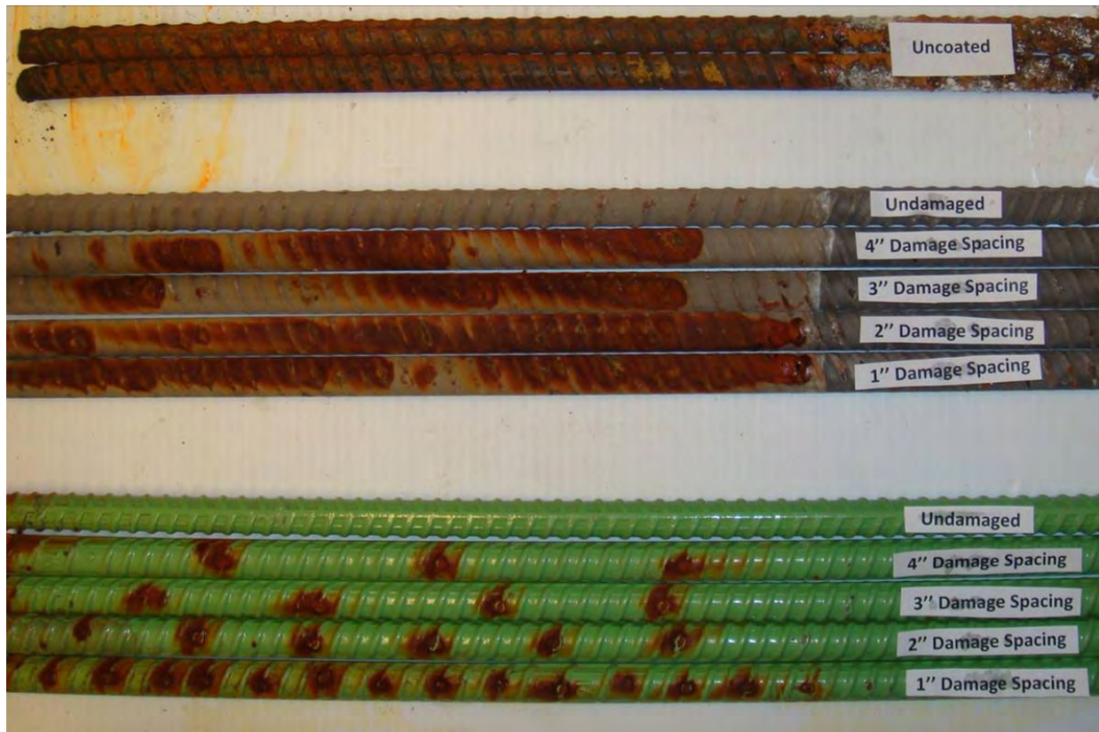
Figure 6.31 Surface conditions of all tested rebar after testing
