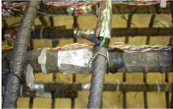
(b) Gauges on main and spiral reinforcement
