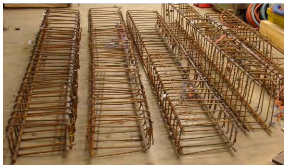
(a) Rebar cage of beams
