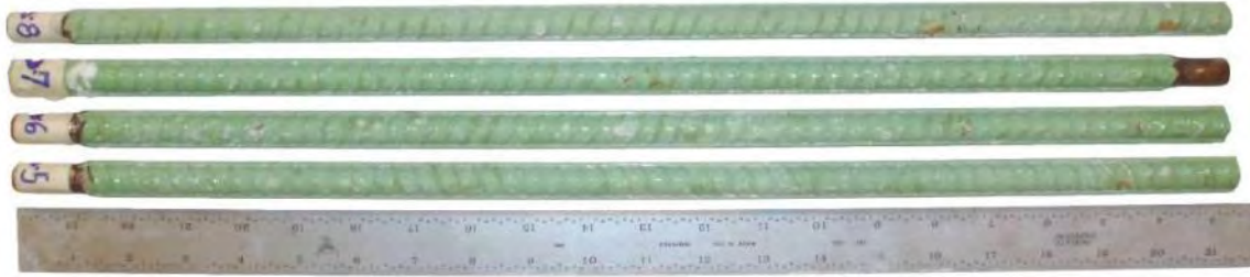
(a) Intentionally damaged epoxy-coated bars removed from a ponding specimen
