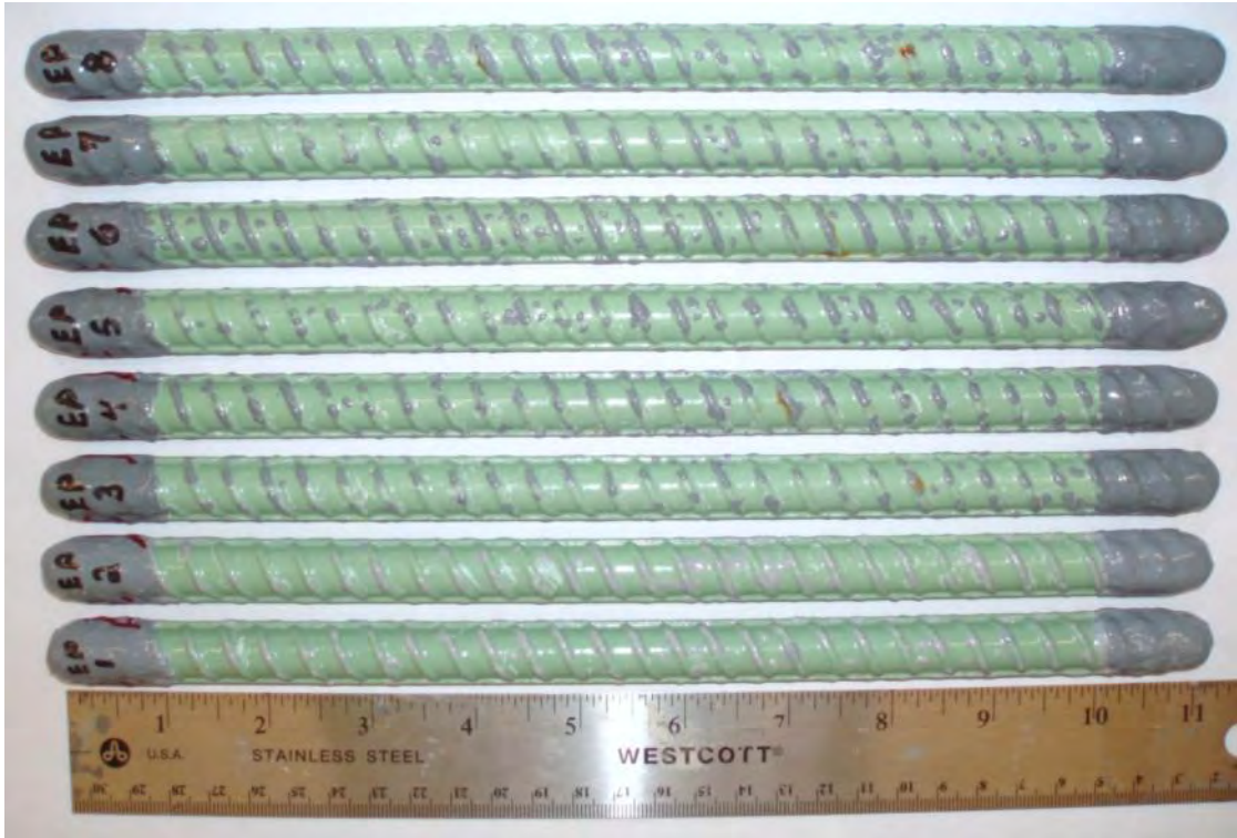
Figure A - 22: Front side of the deformed epoxy-coated salt spray specimens after testing.
