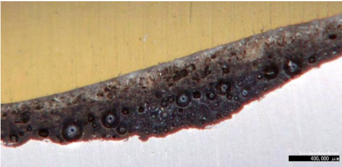
(b) Thick portion of double coating on a deformed rebar showing a distinct boundary
