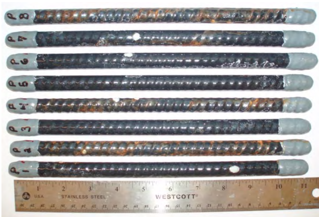
Figure A - 16: Front side of the deformed pure enamel-coated salt spray specimens after testing.
