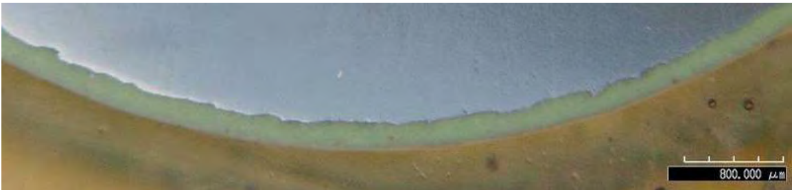
(c) Typical cross-sectional view of an epoxy-coated smooth bar after testing
