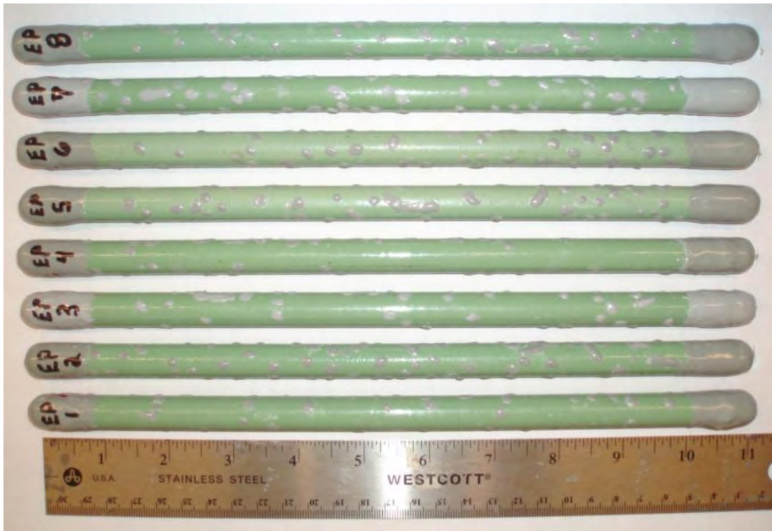
Figure A - 20: Front side of the smooth epoxy-coated salt spray specimens after testing.
