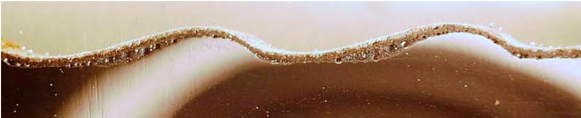
(a) Typical longitudinal view of double coating on a deformed rebar
