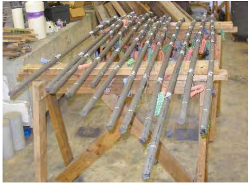
(a) Strain gauges on main reinforcement
