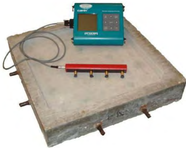
(a) Canin + equipment and the Wenner Probe
