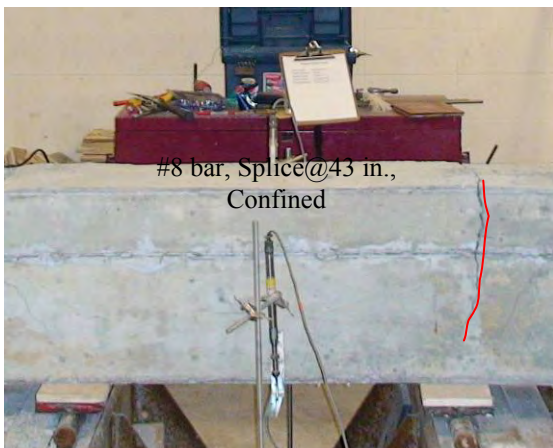
(k) Flexural failure of B-8-3
