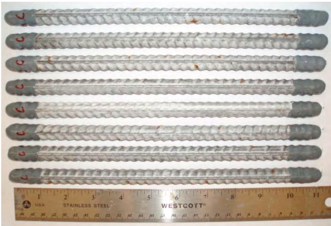
Figure A - 13: Left side of the deformed double enamel-coated salt spray specimens after testing.
