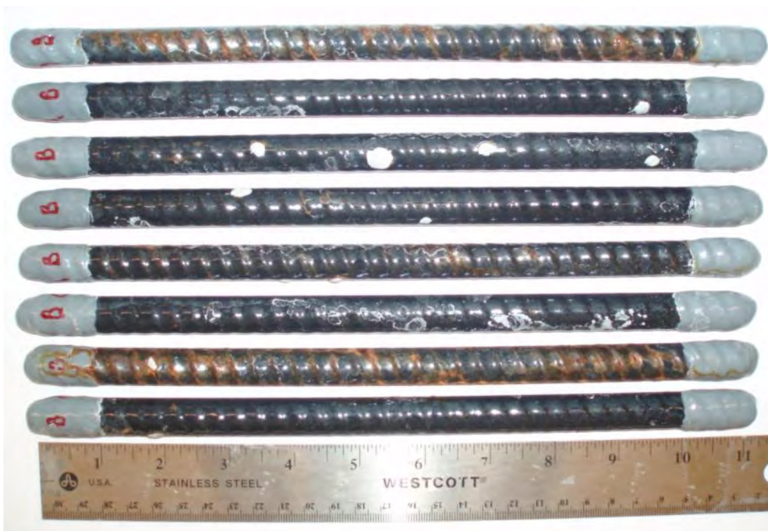
Figure A - 17: Backside of the deformed pure enamel-coated salt spray specimens after testing.
