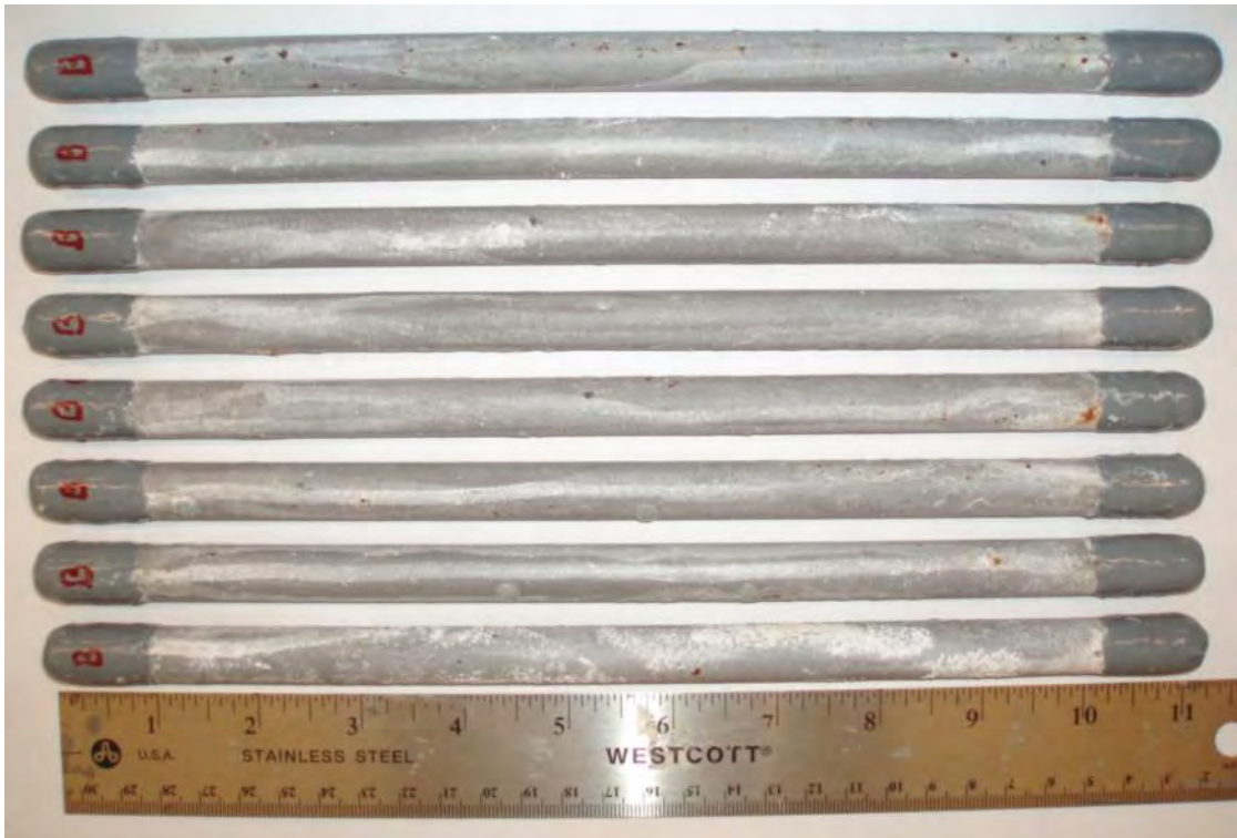
Figure A - 3: Backside of the smooth 50/50 enamel-coated salt spray specimens after testing.
