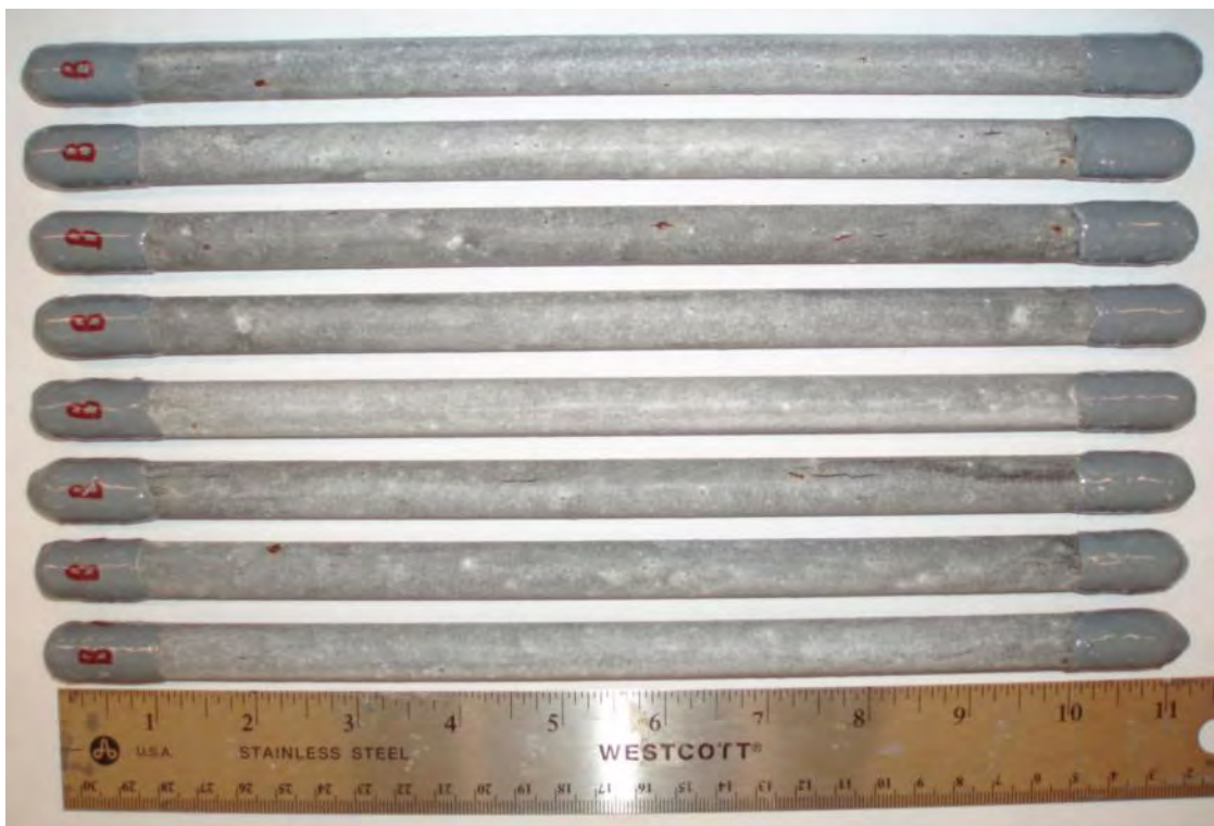
Figure A - 9: Backside of the smooth double enamel-coated salt spray specimens after testing.
