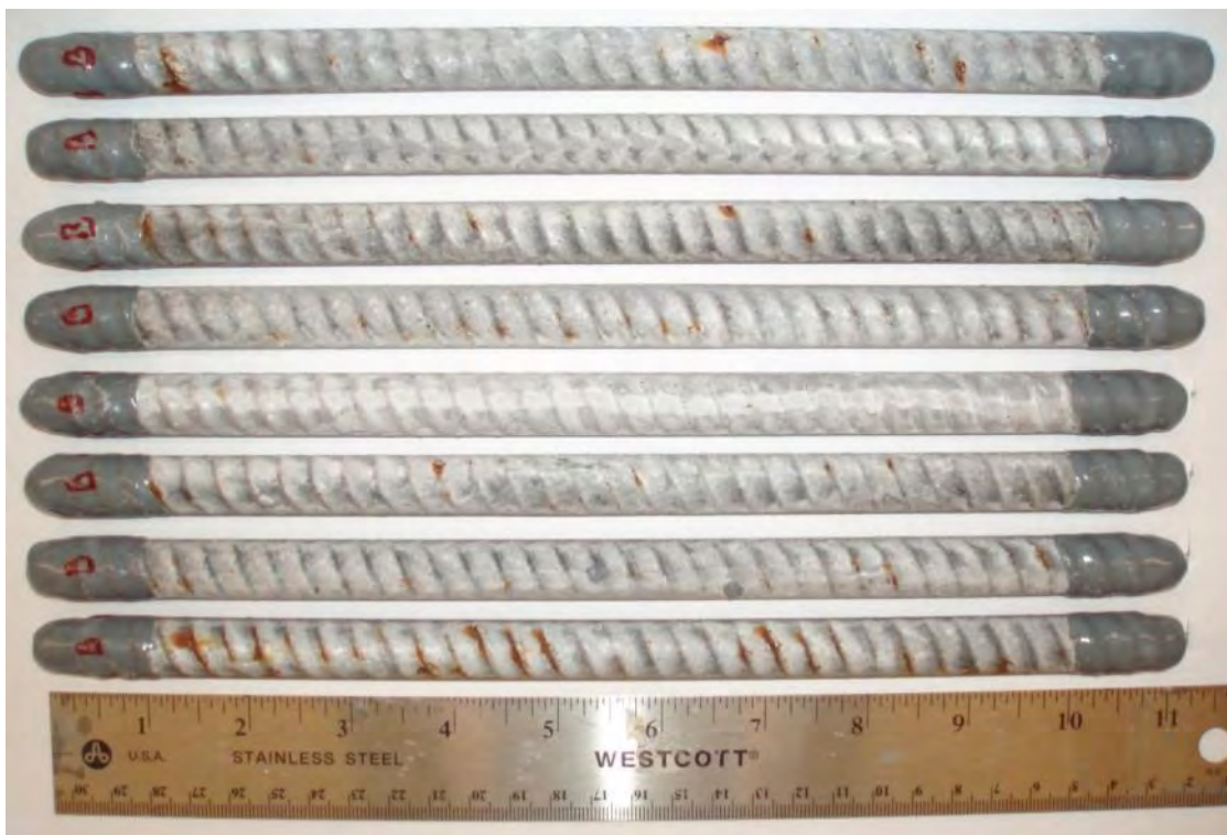
Figure A - 11: Backside of the deformed double enamel-coated salt spray specimens after testing.
