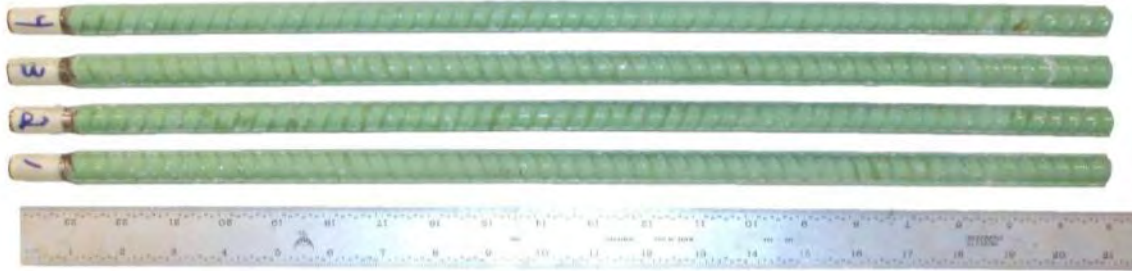
(b) “Perfect” epoxy-coated bars after removal from a specimen
