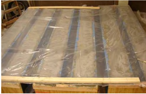
(a) Curing of beams
