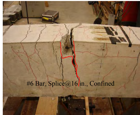
(b) Flexural failure of B-6-2
