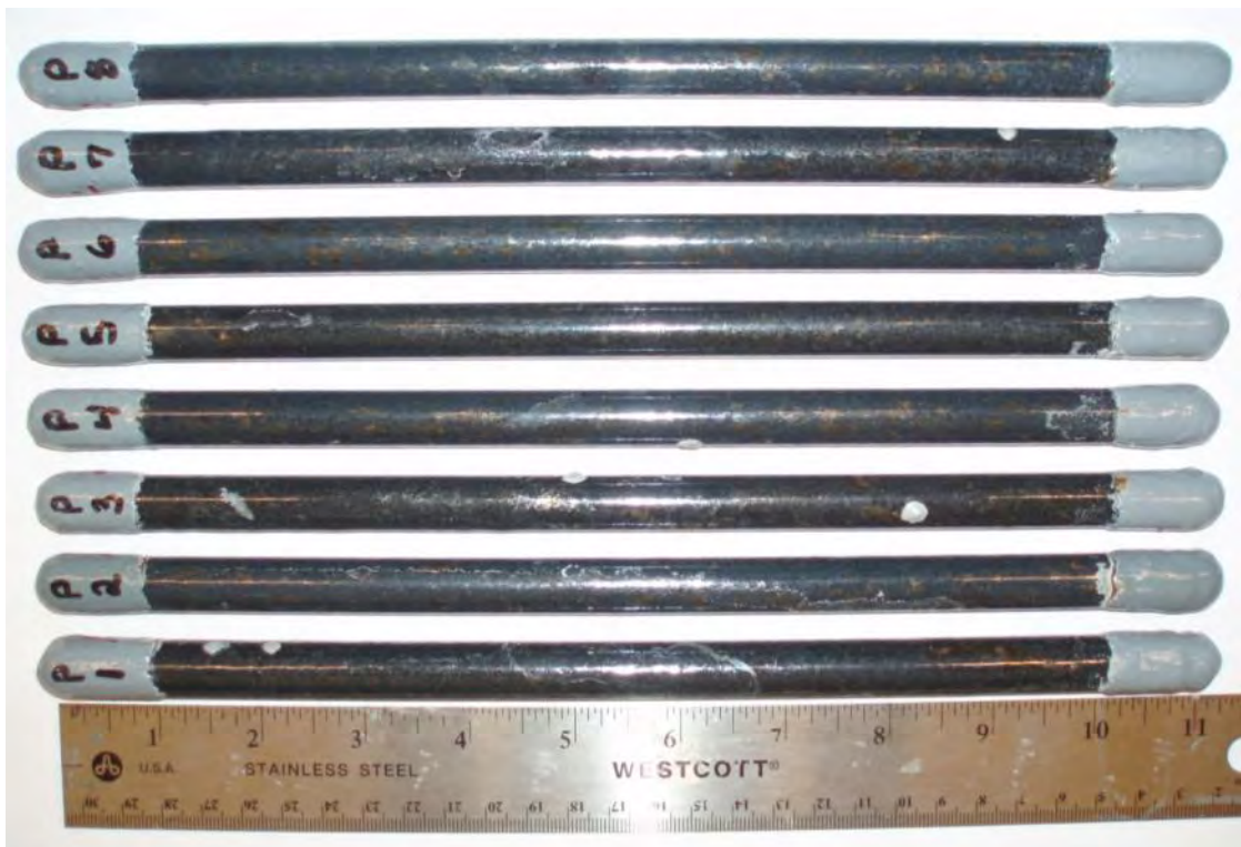
Figure A - 14: Front side of the smooth pure enamel-coated salt spray specimens after testing.
