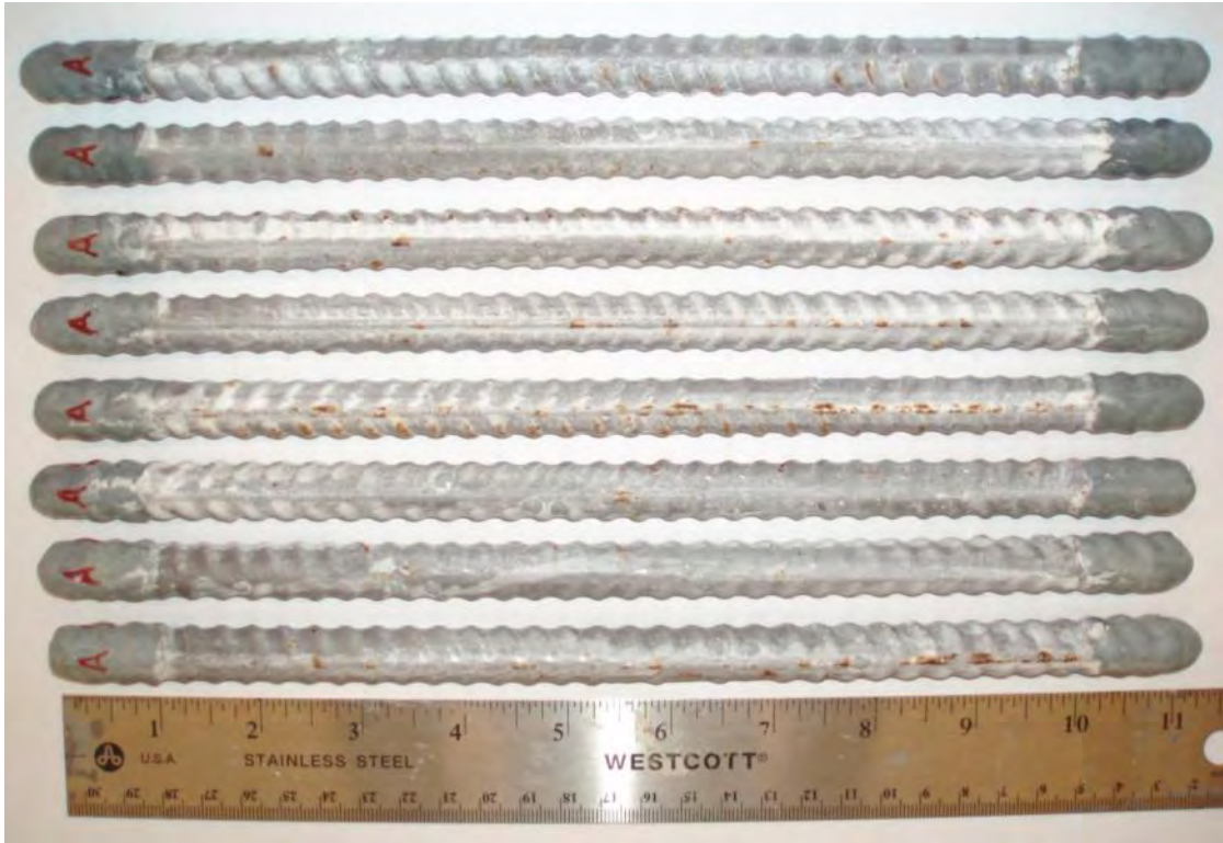
Figure A - 6: Right side of the deformed 50/50 enamel-coated salt spray specimens after testing.
