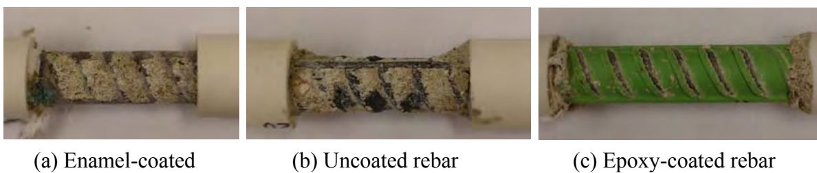
Figure 4.19 Details of concrete-rebar interfaces (#4 rebar).
