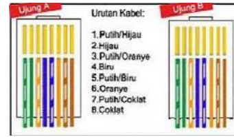
Gambar 2.3 Straight Rrough T568B.
