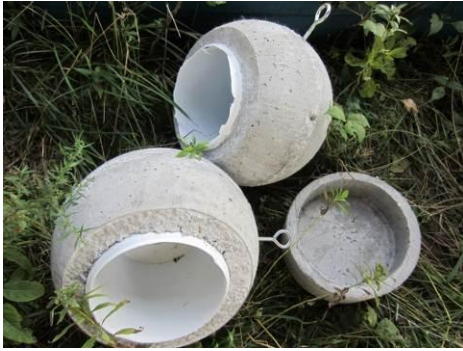
Figure 17. Active Smart Rock concrete shells – base and lid
