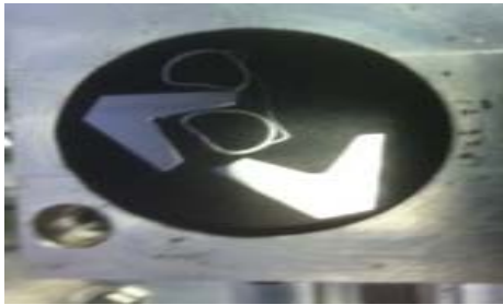
Figure 4. Two “V” shaped samples (one with clip is parent and shiny one is galvanized with coating completely ground off).
