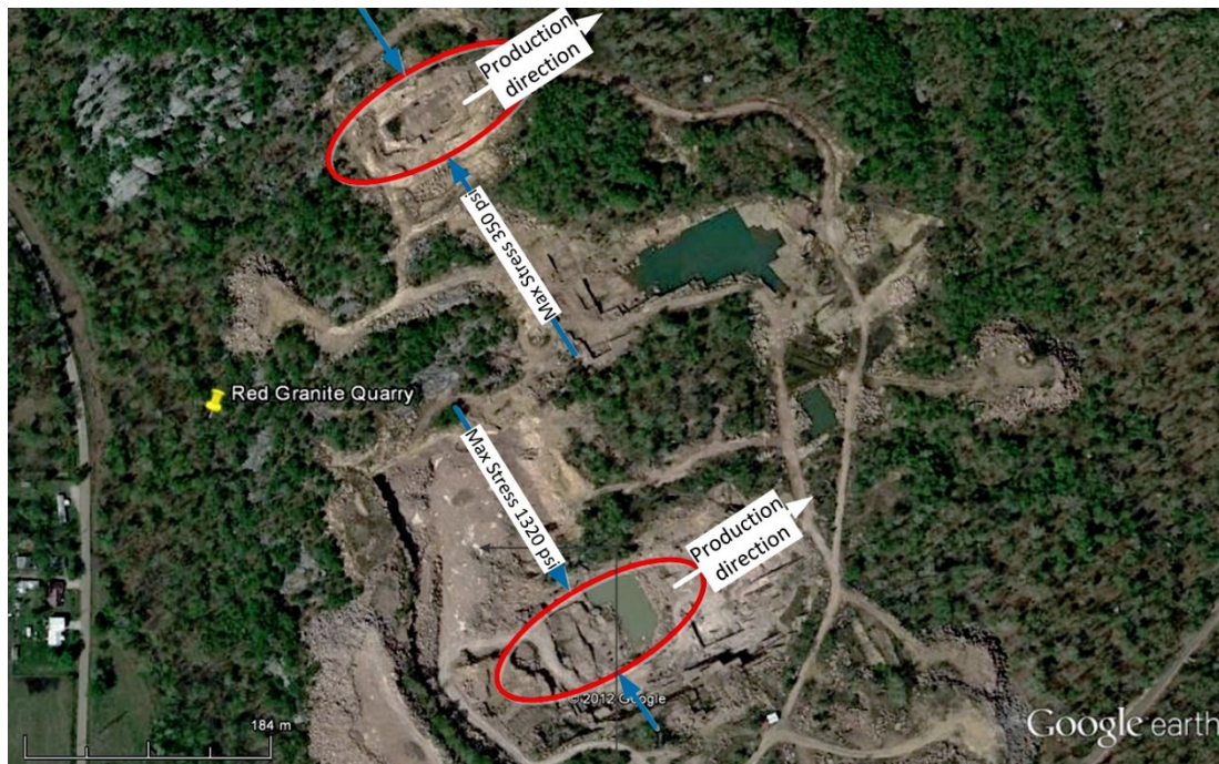
Figure 7 Maximum horizontal stress direction and magnitude
