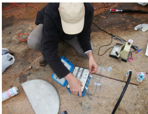
Figure 4. Application of flatjack method in Red Granite Quarry
