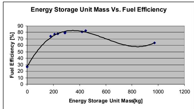
Figure 6. Fuel efficiency as a function of the mass of the energy storage unit
