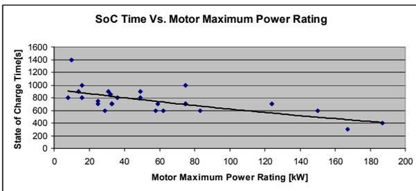
Figure 2. State-of-charge time vs. motor maximum power rating
