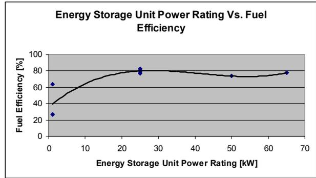
Figure 5. Fuel Efficiency vs. power rating of the energy storage unit
