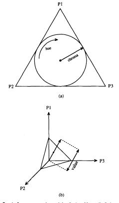
Figure 1. a) Maxwell's Triangle. White is at the center of the triangle. The three primary colors are at the vertices of the triangle. b) An arbitrary color, pictured as a point within the triangle, is defined by its components of the three primaries. These components are obtained by drawing a line perpendicular to the side of the triangle opposite the primary's vertex through the color point. This figure shows the P1, P2, and P3 components as solid lines of the color point.
