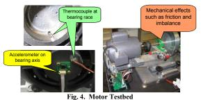
The motor monitoring application will provide remote visibility of power usage and power related health indications, including PF. Additionally, the vibration and temperature measurands are collected to support diagnostics and prognostics of motor and bearing condition. As failures are induced in the
