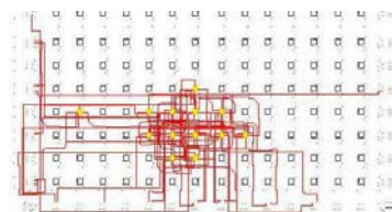
Fig. 3 ALU implementation by mentor graphics using the xilinx XC4000 family of logic gates
