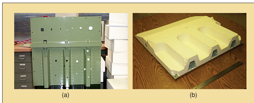
Fig. 9. The SOFI panel picture (a) before (white circles are SOFI void inserts and black squares are rubber inserts) and (b) after SOFI application. From Materials Evaluation , vol. 63, no. 5. Reprinted with permission of the American Society for Nondestructive Testing, Inc.
