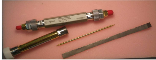
Figure 6. 7/3-mm airlines, a central conductor, and a strip of a flexible magneto-dielectric material under study.
