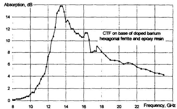
Figure.3. .The dependence of the microwave absorption on the frequency at placing CTF with epoxy resin on the wide wall of rectangular waveguide
