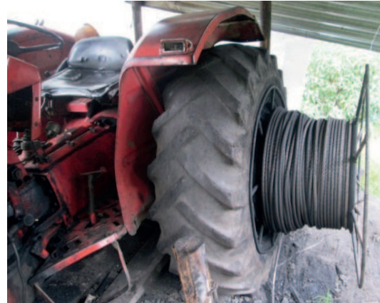
Figure 2. Diesel tractor used for wagon extraction in an underground coal mine.
