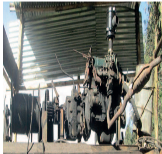
Figure 3. Petrol engine used for car extraction in an underground coal mine.
