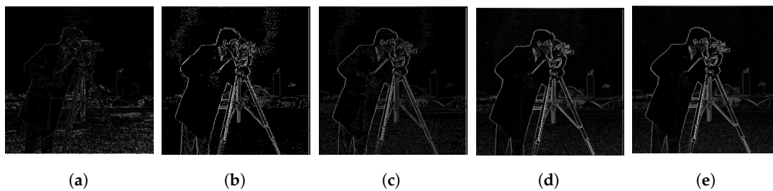
Figure 10. Edge detection using Linear Feedback Shift Registers (LFSRs): (a) eight clock cycles; (b) 22 clock cycles; (c) 64 clock cycles; (d) 128 clock cycles; (e) 256 clock cycles.
