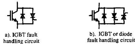
Fig. 4. Suggested power switch modules for fault handling.
