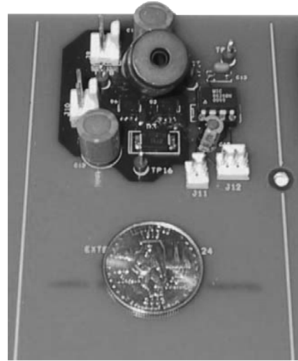
Fig. 2. Photograph of 3-W (nominal) low-input-voltage converter.
