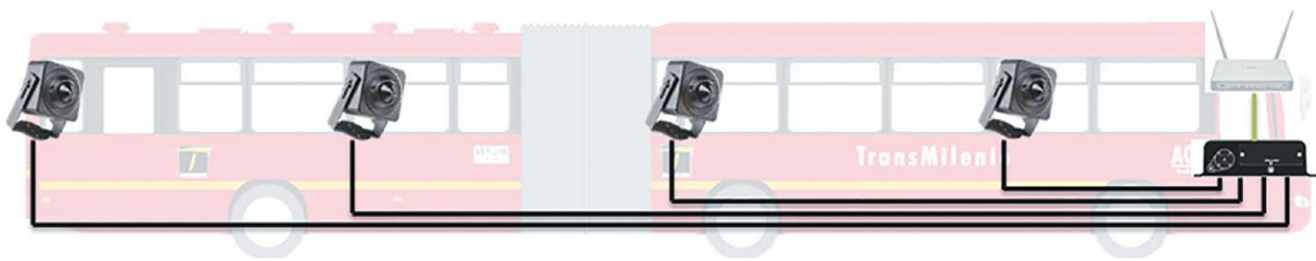
Figure 1. Design installing cameras inside articulated buses
