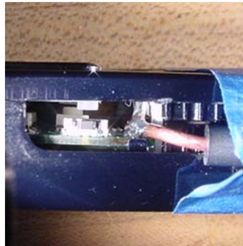
Fig. 10 Side view of the hand held device showing the entry of the coax cable into the player
