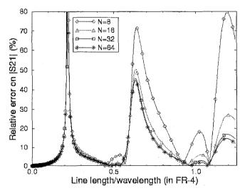
Figure 2. Relative error on |S21| for N=8, 16, 32 and 64.
