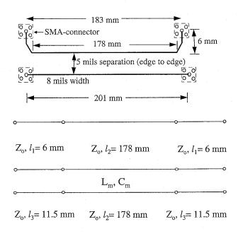
Figure 5. Coupled line dimensions and transmission line modeling.
