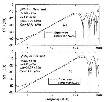
Figure 6. Experimental and simulated result of coupling between microstrip lines with
