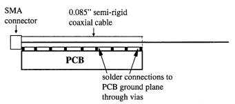
Figure 8. Test configuration for the dipole-type antenna impedance measurement.
