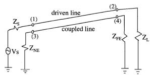
Figure 3. Two coupled transmission lines.
