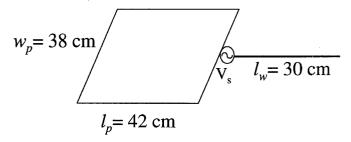
Figure 7. The geometry of the dipole-type EMI antenna.
