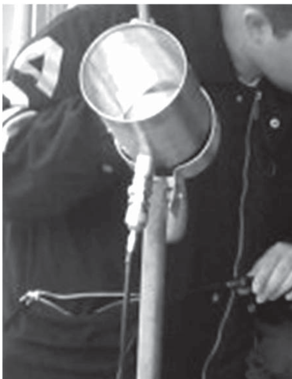
Figure 6. Home-made antenna developed for the Bolivian wireless project
