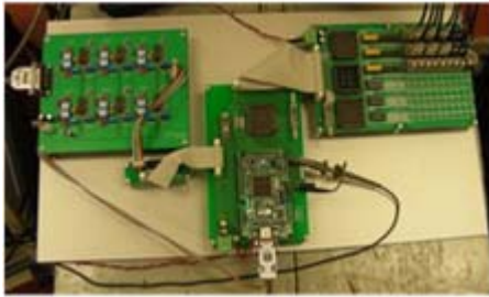
Fig. 4. Experimental Setup for Scaled Model of Hypothetical Ship's Power System [12].
